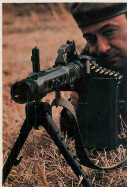
ABOVE: CETME AMELI/MG82 SPAM (Special-Purpose Assault Machine gun) designed by Col. Jose Maria Jimenez Alfaro, director of CETME, shows distinct likeness to MG42. LEFT: CETME MG82 in Cal. 5.56mm NATO shown with 200-rd. assault pack.
